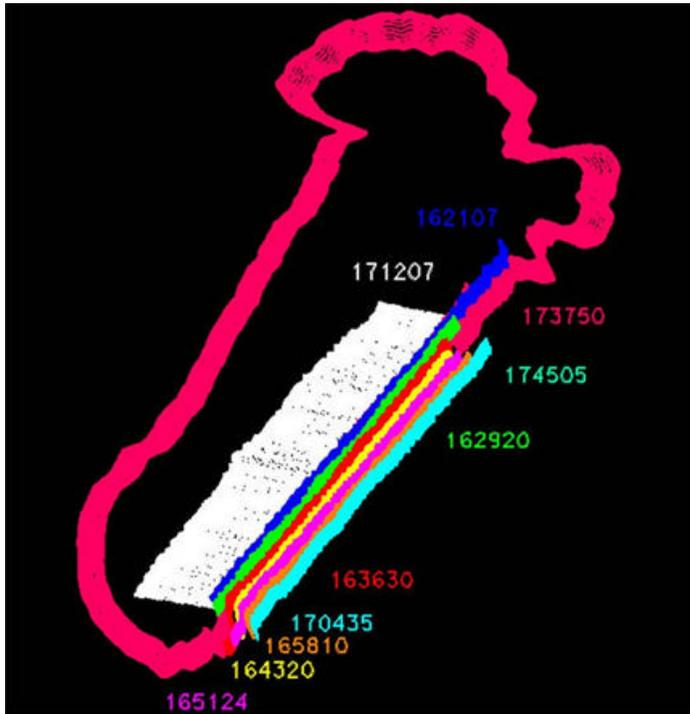
Figure 3. This illustrates an immediate data collection validation procedure, which converts a portion of the LIDAR points to a raster file for display using GIS software. Note that the scanner was not disabled while the aircraft turned (pink flight line) showing the complete flight path for this single pass.
